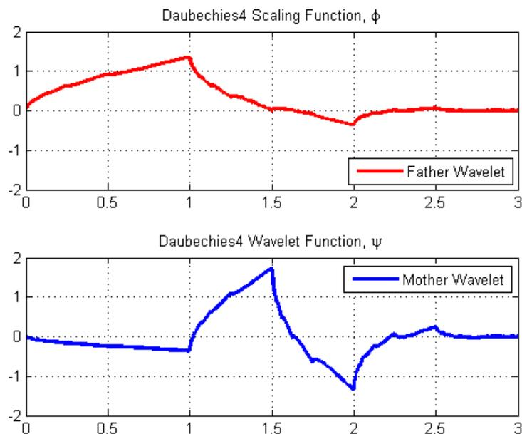
**Figure 3:** Daubechies-4 Wavelet's Scaling Function and Wavelet Functions plotted.
