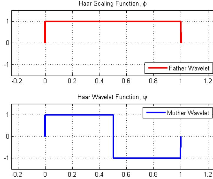
Figure 2: Haar Wavelet's Scaling Function and Wavelet Functions plotted.
