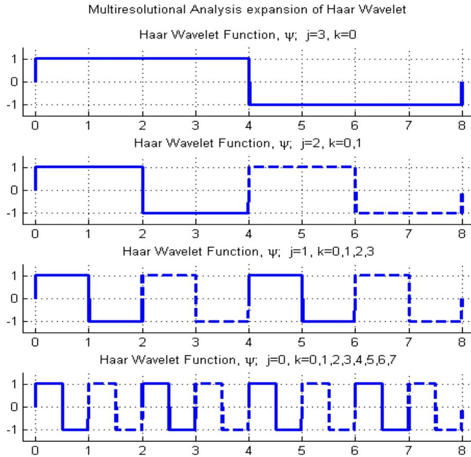
**Figure 1:** Multiresolutional Analysis expansion of some possible  $j, k$  values and their corresponding windows of analysis through the Haar Wavelet.
